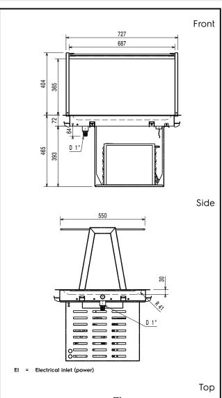
Electric Supply voltage: 220-240 V/1N ph/50 Hz Electrical power, max: 0.47 kW Water: Water drain outlet size: **Key Information:** External dimensions, Width: 770 mm 620 mm External dimensions, Depth: External dimensions, Height: 794 mm Net weight: 50.76 kg Shipping weight: 74 kg Shipping height: 1060 mm Shipping width: 660 mm Shipping depth: 810 mm 0.57 m<sup>3</sup> Shipping volume: -10 / 0 °C Set temperature: -10 / 0 °C Top temperature: **Refrigeration Data** R290 Refrigerant type:
